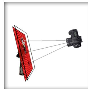
If your lens is set to a small aperture it may provide enough depth-of-field that this backwards shift in focus may not be apparent. On the other hand, if your lens is set to a large aperture ( $f/2.8$  or
