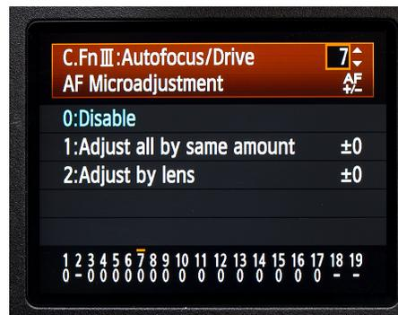
Many professional and semi-professional EOS DSLRs therefore have a built-in micro-focus adjustment feature. This is a Custom Function (C.Fn) that allows you to precisely adjust the focusing tolerances of a particular lens (or set of lenses) to match those of your camera body.
